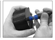
In the «GAS» slot, insert the blue connector (under the casing, on the right side).
