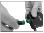
Then connect the other part of the connector to the sensor.
