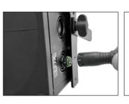
In the «LUX» slot, insert the black connection (on the right side).
