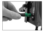
In the «DUST» slot, insert the green connection (on the left side).
